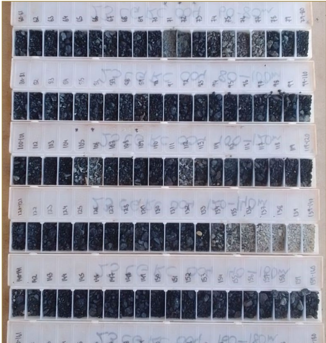
Figure 3: RC chips of in-situ nickel-sulphide style mineralisation in mafic/ultramafic units.
