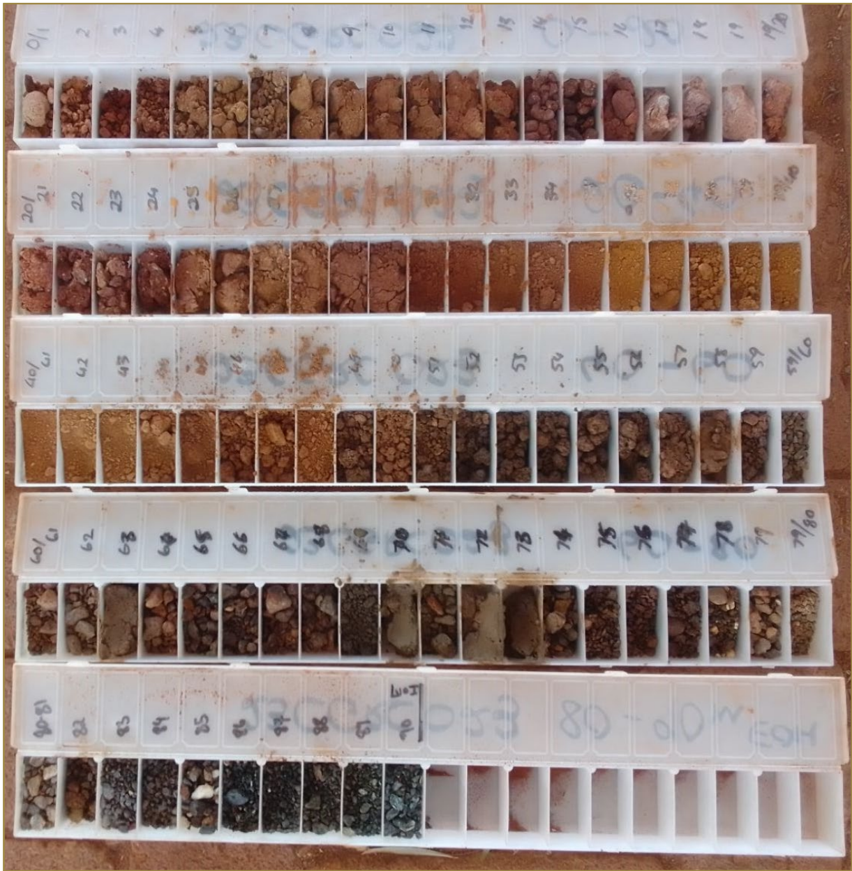
Figure 2: RC chips of laterite style mineralisation, going into the mafic unit at the end of the hole.
