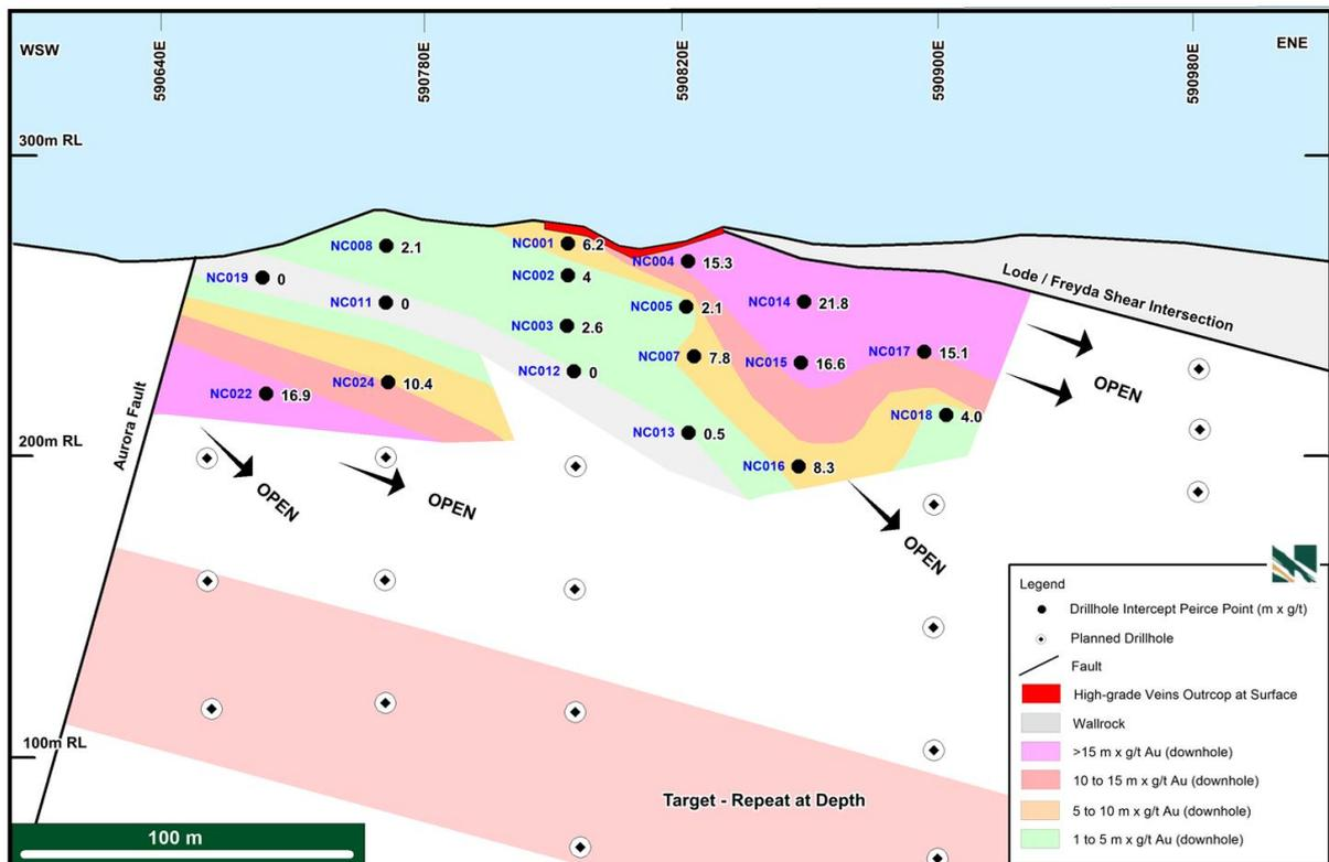
Figure 4: Nunyerry North long section (looking NNW) showing m x g/t Au (downhole width) for the Main Lode #1
