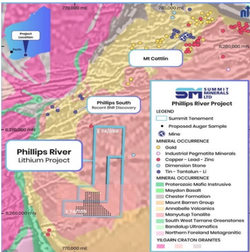
Figure 2 – Proposed Auger Drilling Program at Phillips River Lithium Project.
