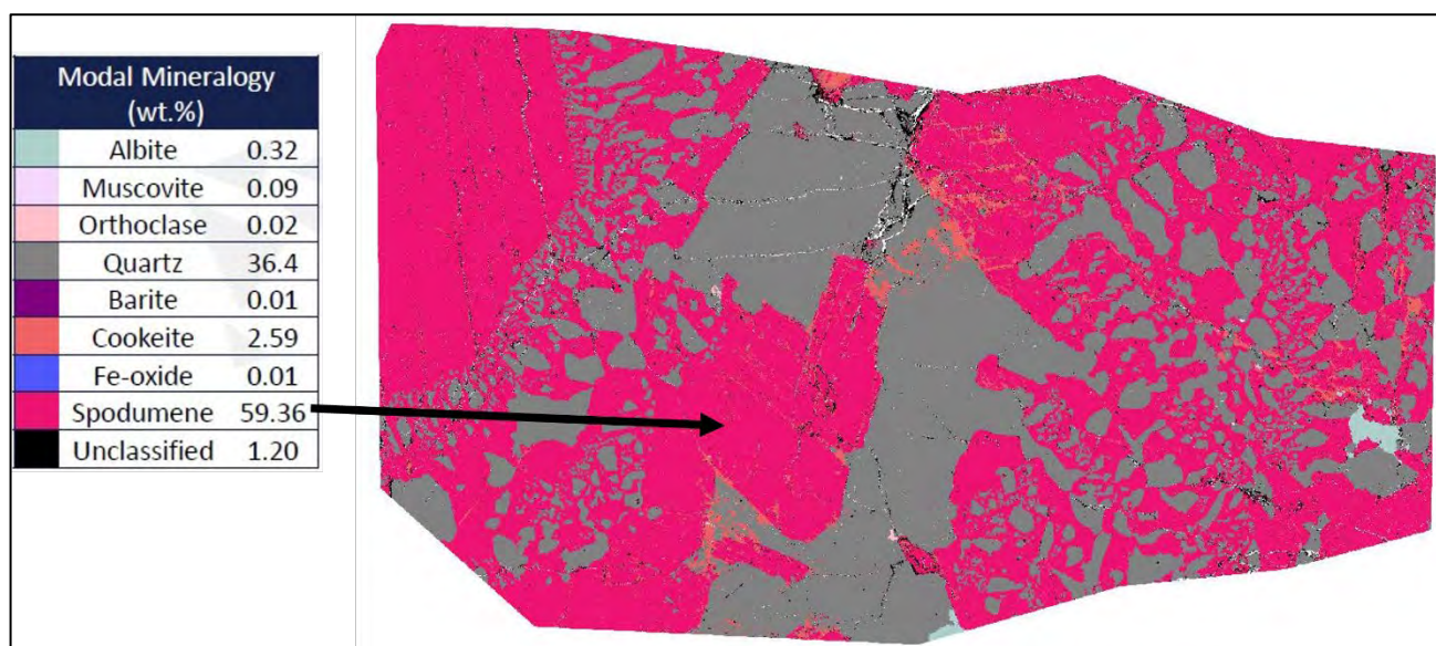
Figure 19: SEM image of Spargoville rock chip sample (Sample ID. KCSA039, see Figure 18 for location) Spodumene is denoted by the pink coloured mineral comprising approximately 60 weight % of the sample (courtesy: RSC Mining and Mineral Exploration)
