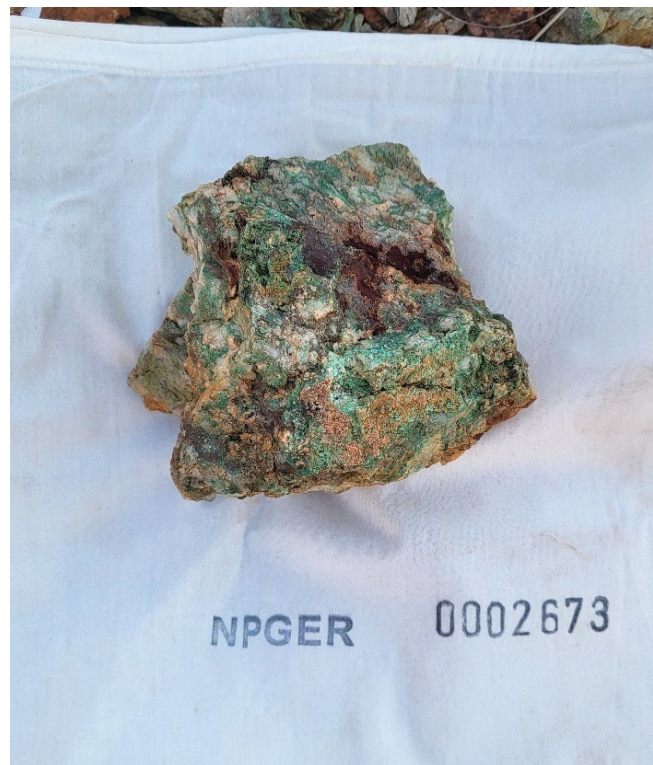
Figure 1: Historical workings at Feral Cat (left), between Tombstone and Belvedere, and sample NPGER0002673 from same location (right), which returned 4.31g/t Au and 6.09% Cu
