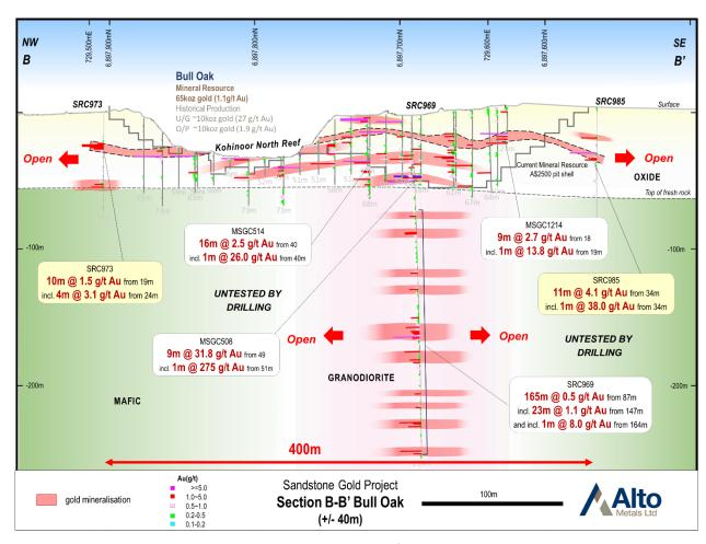
Figure 1: Drill section at Bull Oak looking north-east, showing two of the shallow step-out holes outside the intrusion and the multiple stacked lodes below the open pit and current mineral resource.
