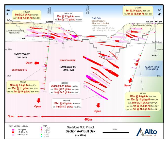
**Figure 5**: Drill section at Bull Oak looking north-west, showing two of the completed deeper drill holes (SRC969 and SRC971) to test extensions of the multiple stacked lodes below the open pit and current mineral resource.
