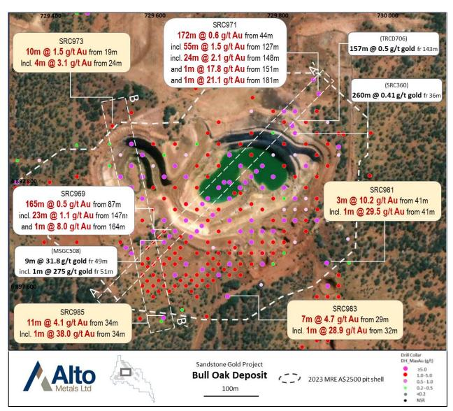
Figure 2: Plan view of Bull Oak Mine showing historical and Alto Metals drilling.
