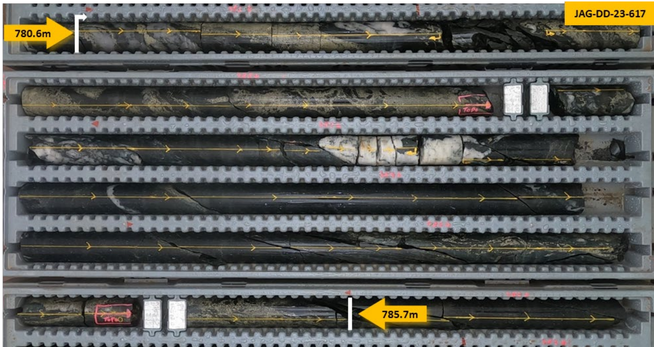
Figure 5 – Core photo from drill hole JAG-DD-23-617; 780.6m to 785.7m down-hole: Stringer, semi-massive and massive sulphides (metallic bronze) mineralisation with dacite host rock.
