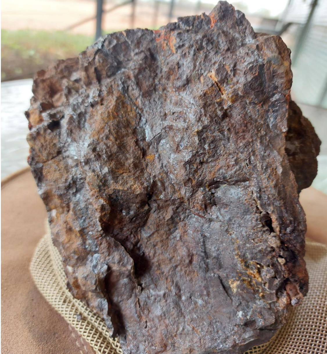
Figure 6: Photograph of the massive ironstone found at the Candy Colette Anomaly with abundant manganese and specular haematite. Estimated abundances of specular haematite are 45% and manganese 3%, all disseminated within the rock matrix.
