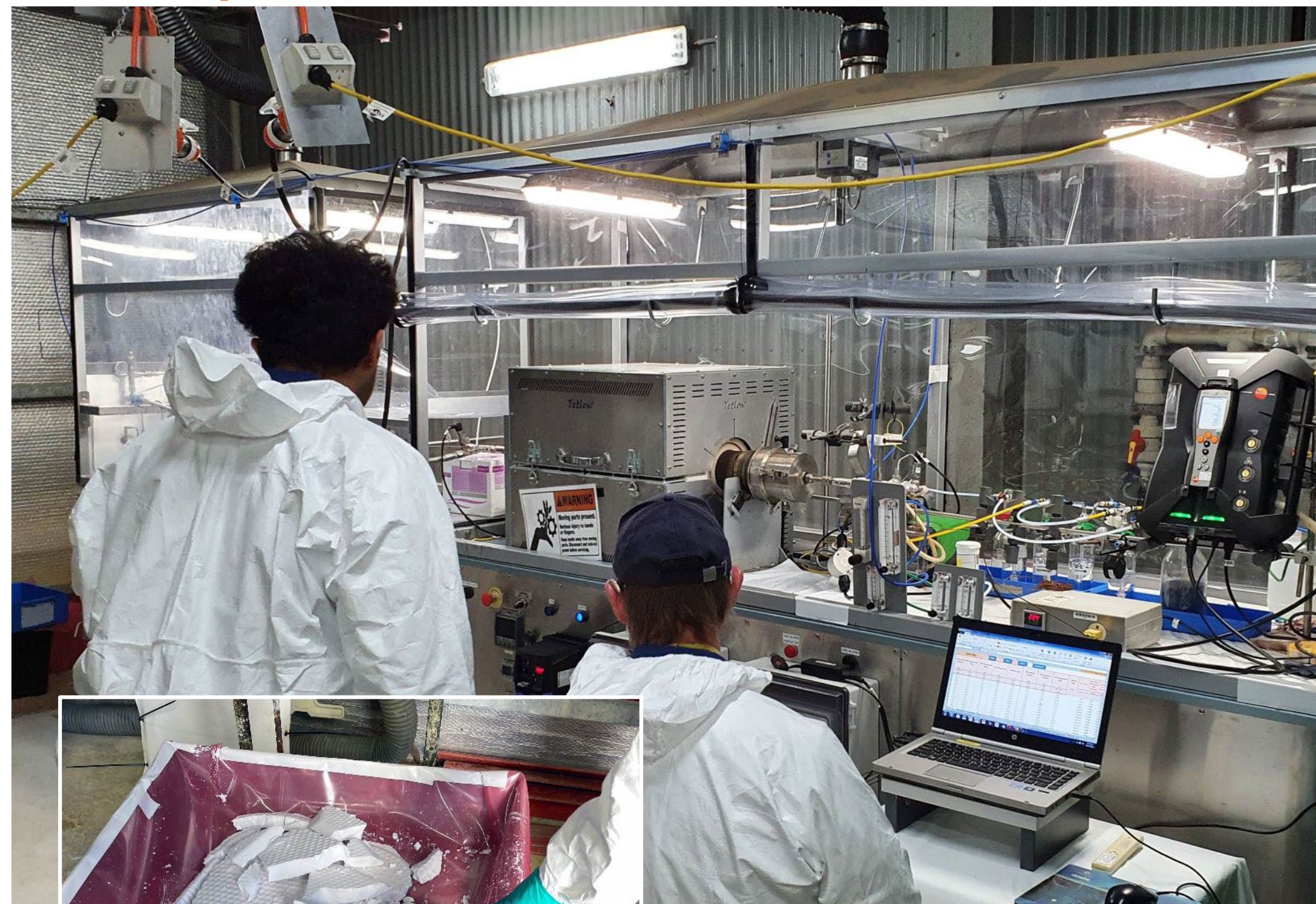
Above: Goschen's rare earth product undergoing bench scale sulphation kiln testwork at ANSTO.
