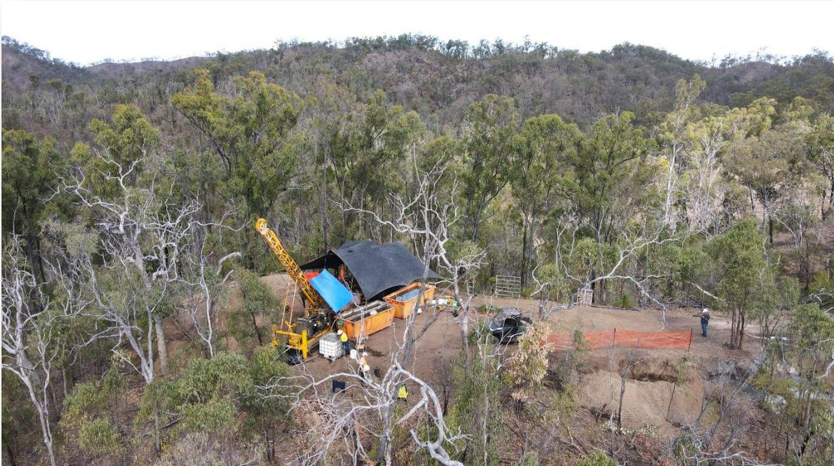
*Figure 6. Core drilling at Briggs Central.*
