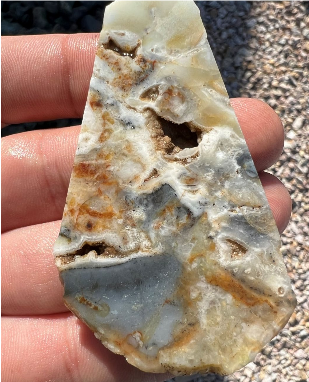
Figure 2: Sample 1671147 from the Calico Silver prospect which returned 678 g/t silver.
