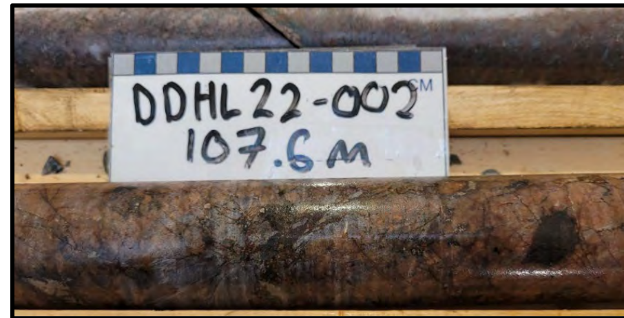
Visible uraninite from S-Zone drill hole
