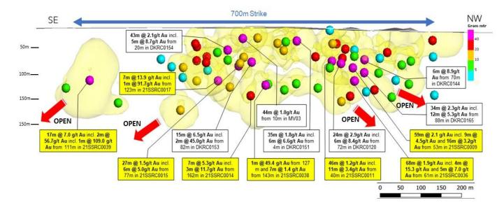
Long Section of the Southern Star mineralisation showing selected gold intercepts. Mineralisation remains open in nearly every direction including down-plunge, down-dip and along strike to the north and south.
