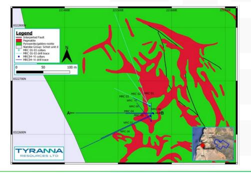
Location of RC drill-holes MRC01-MRC10. Note location of cross-section A-B
