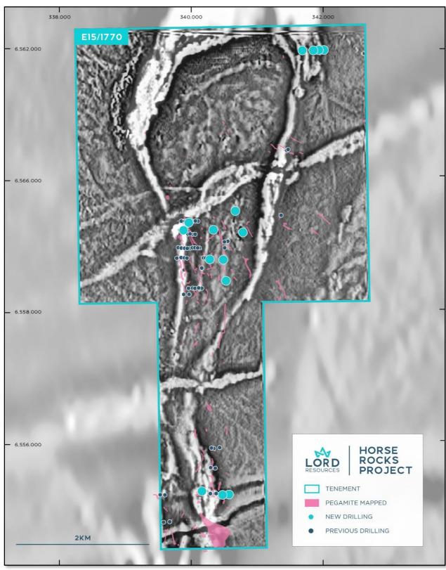
Figure 2 Drillhole location plan overlying drone magnetics
