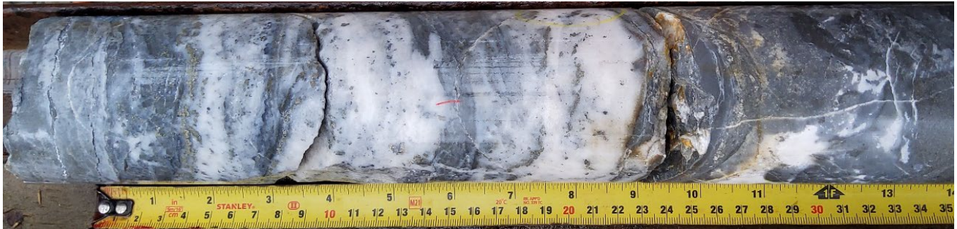
Plate 2: Drill hole PPDD23-001 epithermal vein intersected at 66.37m
