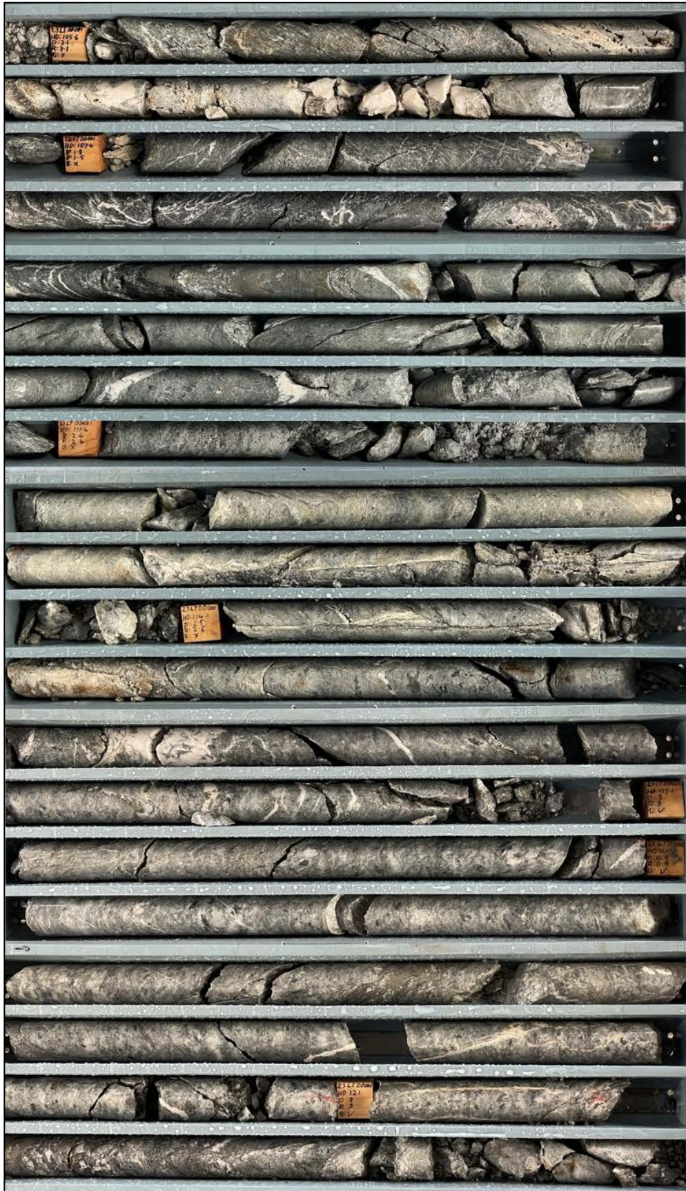
Figure 7: 23LTRD001 from 105m to 122m downhole. The interval is foliated, locally brecciated with dominantly barite fill.
