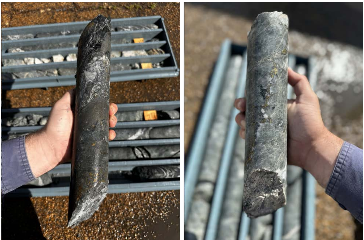
Figure 1: Drill core from 23LTRD001 showing chalcopyrite, sphalerite and barite at 109.3m (left) and chalcopyrite within a heavily silicified and brecciated volcanic at 116.4m (right). Summary log with sulphide abundances in Appendix C.
