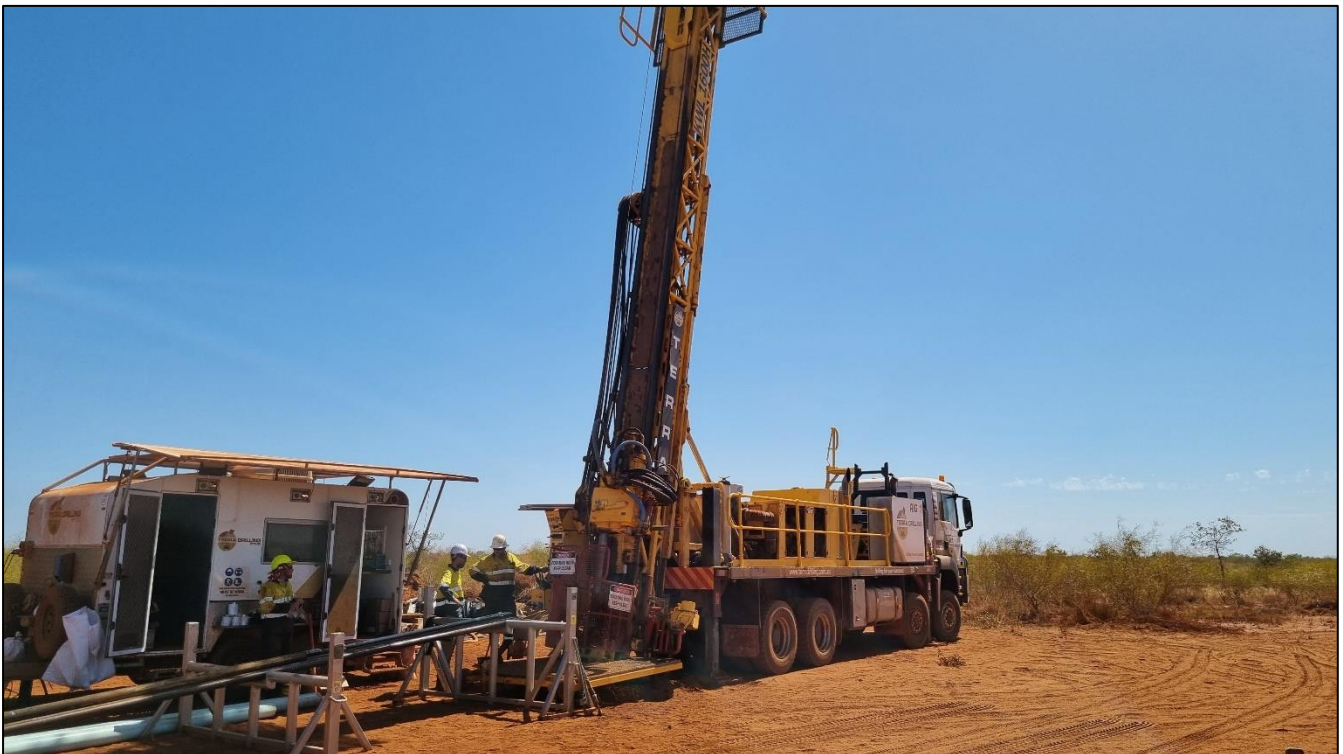
Figure 1. DD drill rig set up on the first hole at Coral Bug IOCG target.
