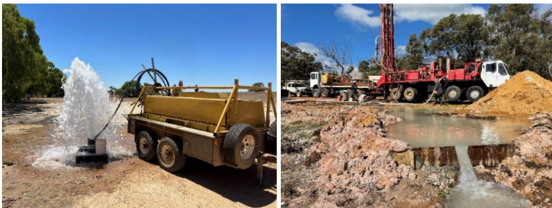
Figures 3 & 4: Variable rate test pumping and monitoring as part of the field program for numerical groundwater modelling and licencing assessments.
