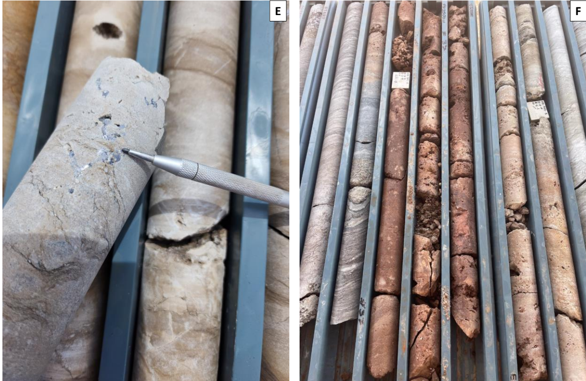
Figure 4, Part 3: Geological, textural and alteration variability of logged geology showing: (E) Galena-filled voids at 304m, and (F): Strong to intense iron-oxide alteration with complete obliteration of host rock. The alteration seems to mark a transition from vuggy dolomitic siltstone with patchy-carbonate infill to laminated shale with minor sandstone interbeds.
