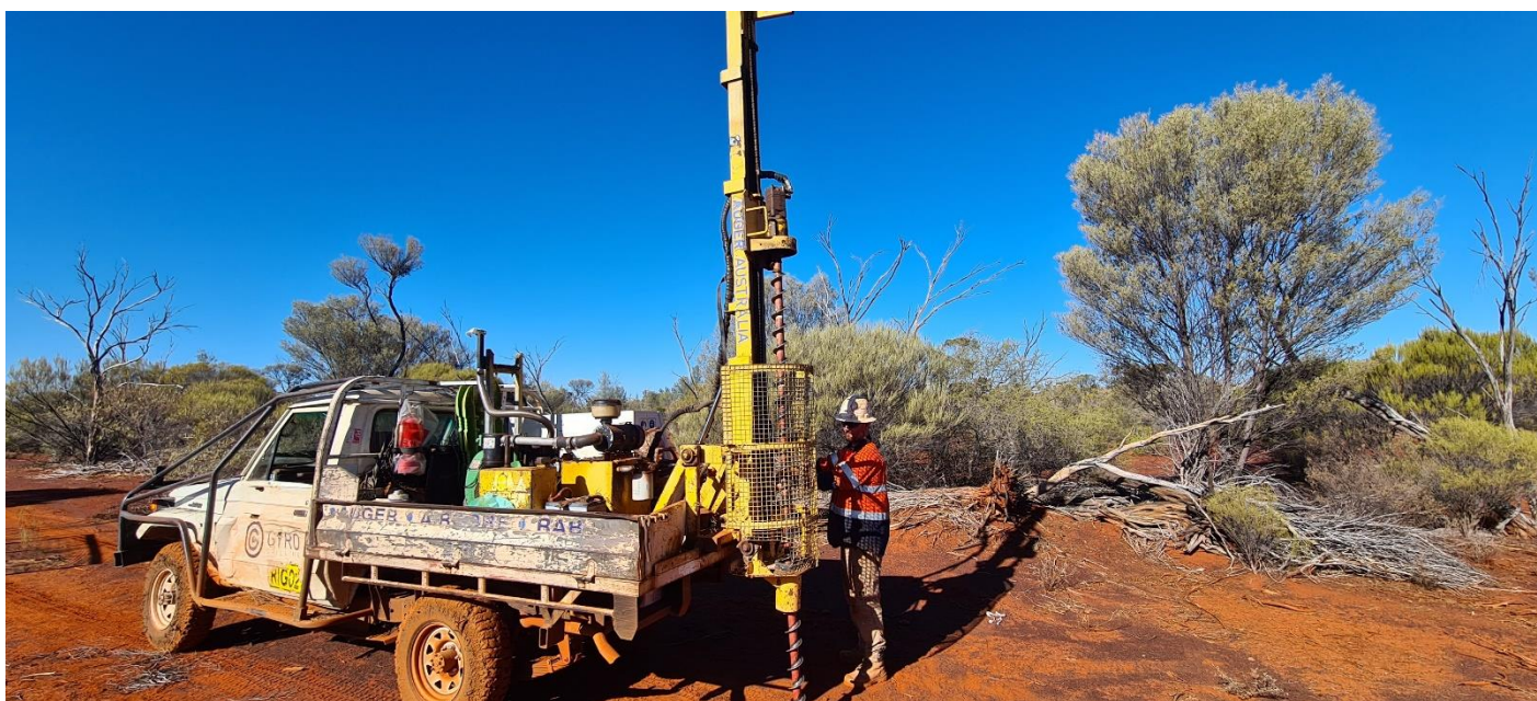
Figure 3: Gyro Australia Auger drill rig commencing auger drilling at the First Hit Gold & Lithium Project.
