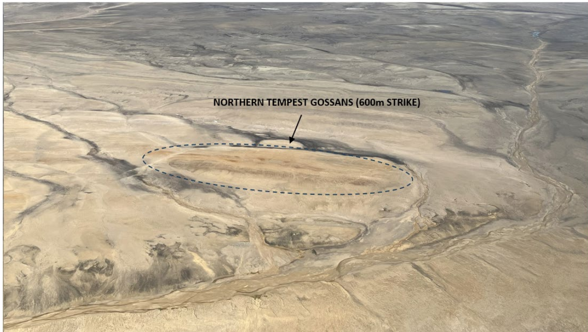
Figure 2: Aerial view of the northern gossan at the Tempest Prospect. This section of the prospective trend has outcropping gossans that can be traced for 600m (brown-rust coloured).
