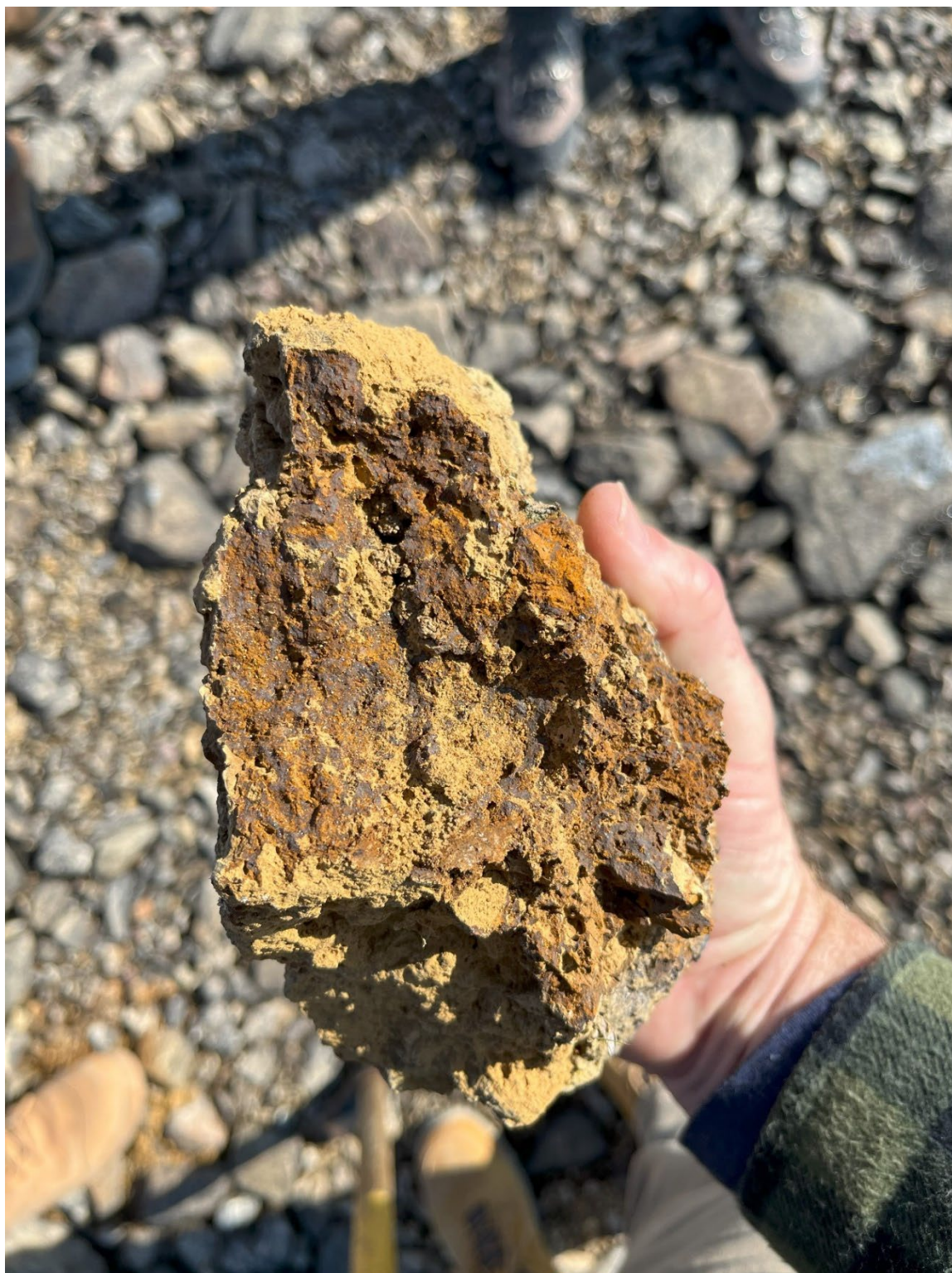
Figure 1: Zinc and lead-rich gossan in outcrop from the Tempest Prospect, Storm Project, Nunavut. Sample ID Y010803.
