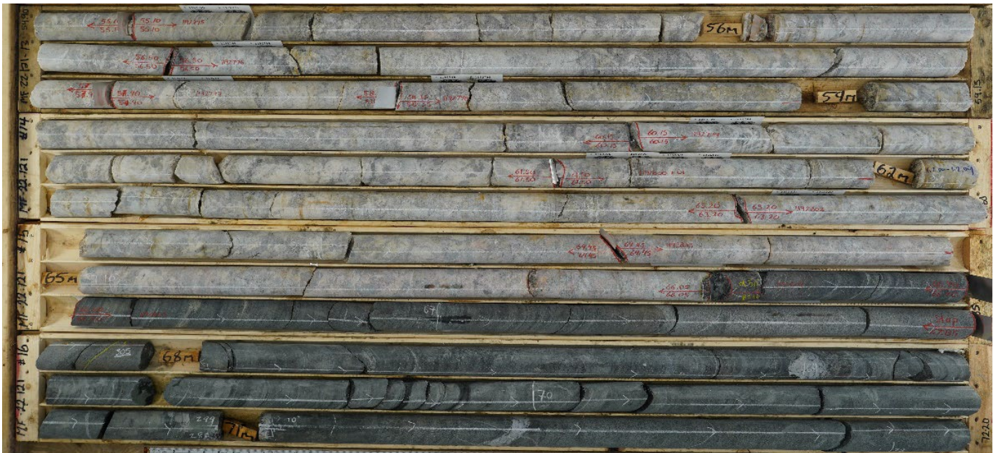
Figure 1 – Section of core from drill-hole MF22-121 showing waste rock (dark) and pegmatite (white).
