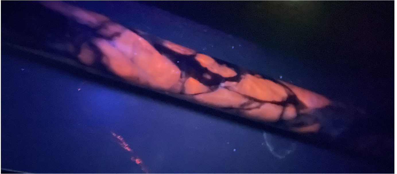
Figure 2 – Section of core from drill-hole MF22-107 showing the UV response of spodumene (orange) within pegmatite.
