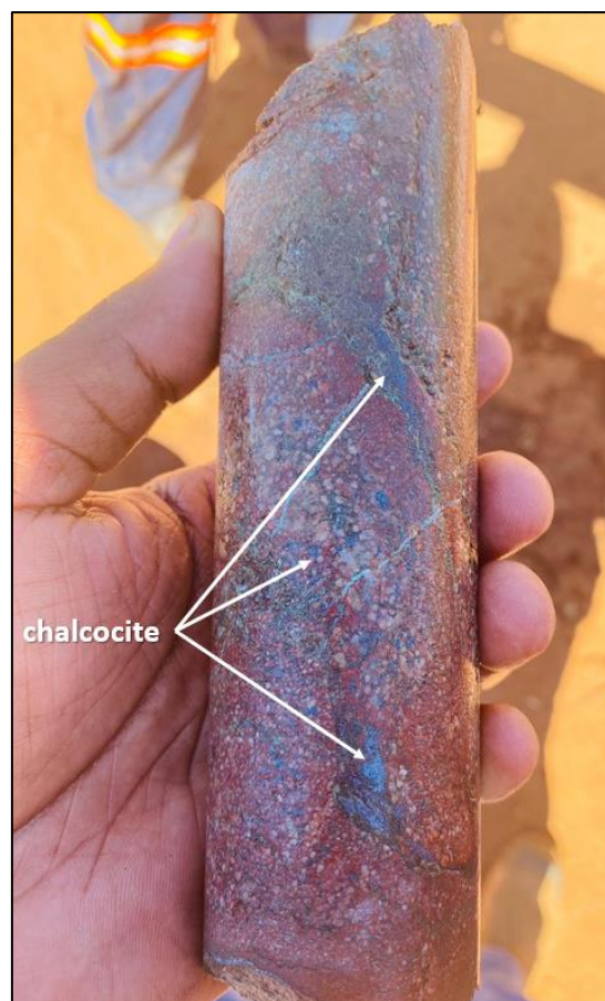
Figure 1: Chalcocite disseminations and veinlets (metallic grey) in weathered biotite schist DBRD149 between 39.55 – 41.47m down hole.
