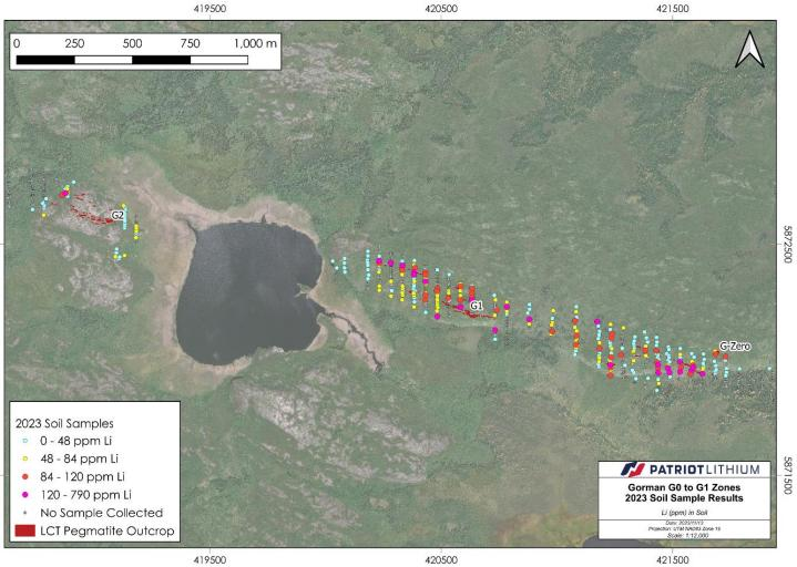
Soil samples taken along and across the high grade G0, G1 and G2 LCT pegmatite outcrops at PAT's Gorman project, and their interpreted extensions under soil cover, have returned highly anomalous lithium values.
