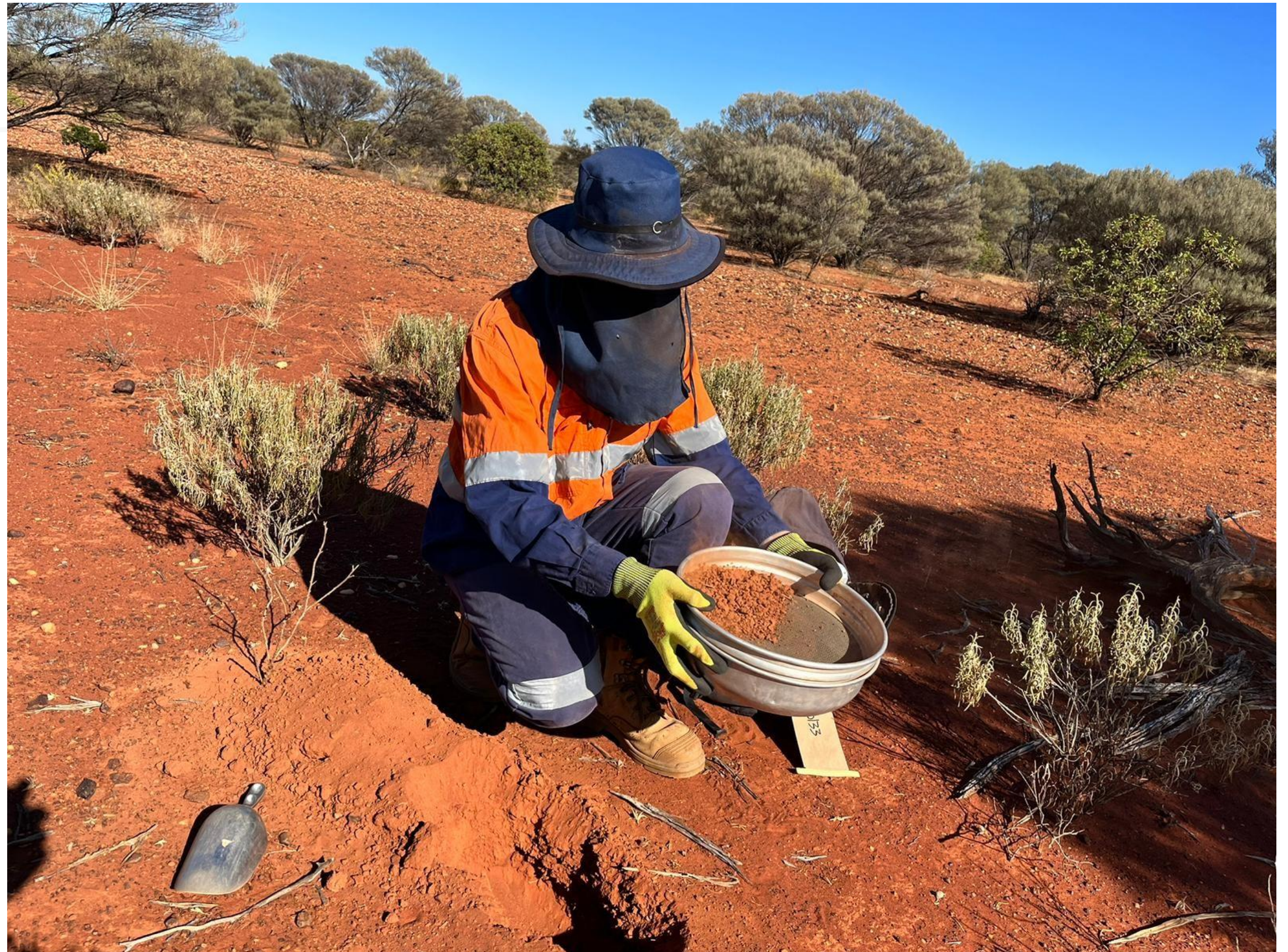
Orientation soil geochemical sampling to assess lithium potential: Ironstone Well - Barwidgee
