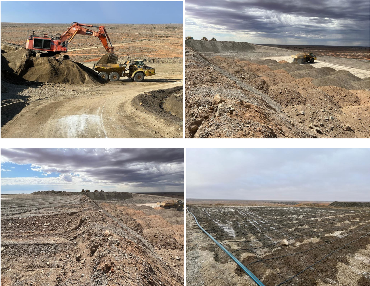
Figure 1: Stacking new cells with mineralised material and irrigation underway on the first and second new cells, which will support increase gold production
