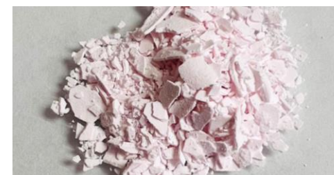
Image: a photo of a >99.9% pure, battery grade Mn sample produced from Tshipi ore, using Jupiter's own production process
