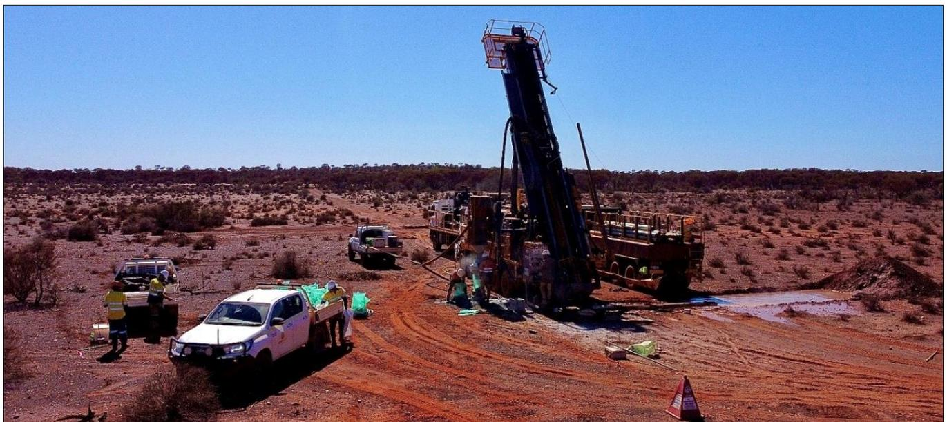
Figure 1 RC drilling rig on site at Guyer North - West.
