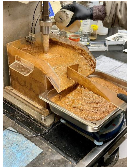
Figure 9: Successful froth flotation test on the Yin bulk sample.
