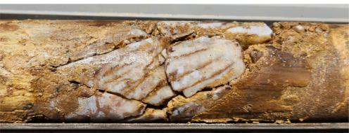
Core sample from diamond drill hole 23YJDD217 between 17.70 and 17.89m showing iron-rich quartz veining.
