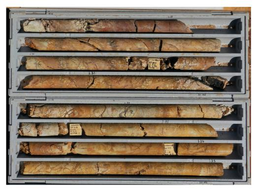
Trays 9 and 10 of diamond drill hole 23YJDD219 between 28.35 and 35.06 m depth. Veining and structural deformation have been logged throughout the entire section (see Appendix B for details).
