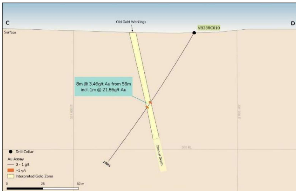
Figure 19. Victor Bore Project Cross Section C-D
