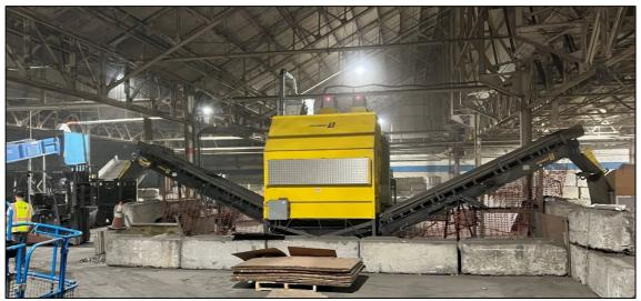
*Figure 3 – Steinert Multi-Sensor Sorter Testing Oracle Ridge Samples*
