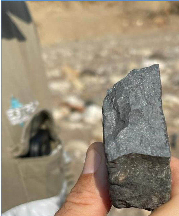
Figure 4: Platy Pyrolusite forming >90% of the specimen found during field reconnaissance to the Mining Concessions
