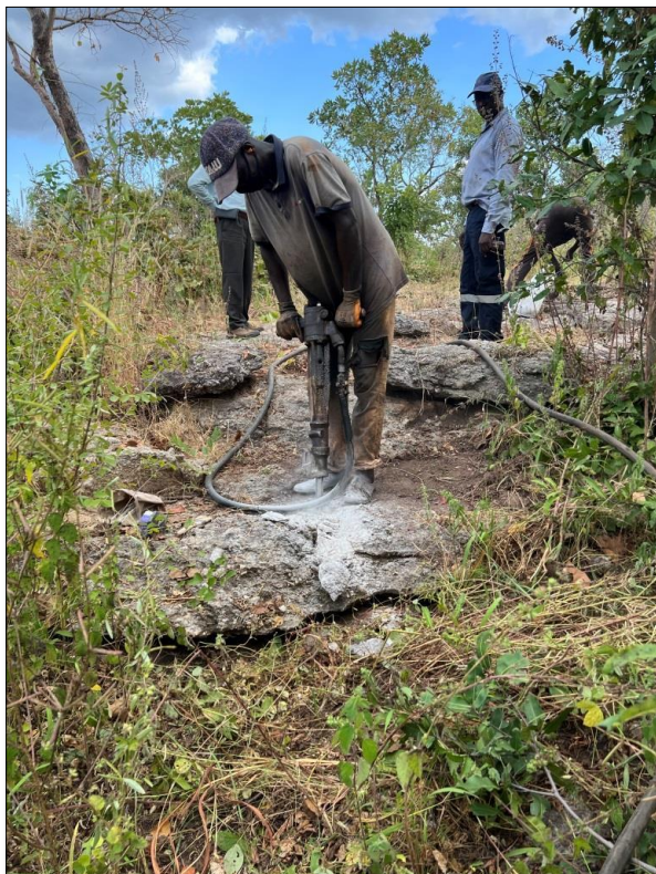
Figure 2: Channel sampling taking place in outcrop sample line BCH02_West.
