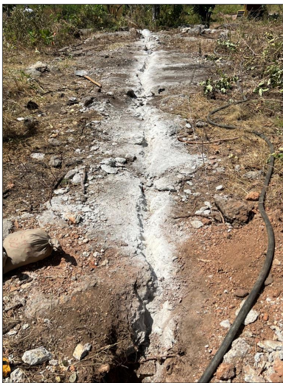
Figure 2: Channel sampling taking place in outcrop sample line BCH02_West.
