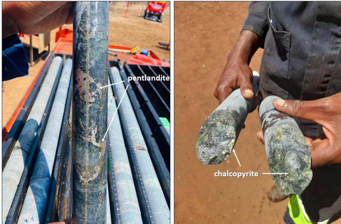
Figure 1: Ni and Cu sulphide examples. Left: Pentlandite semi-massive texture in amphibolite in MARD160 at 208.11 – 208.70m. Right: Chalcopyrite veinlets logged in MADD155 at 187.50m.
