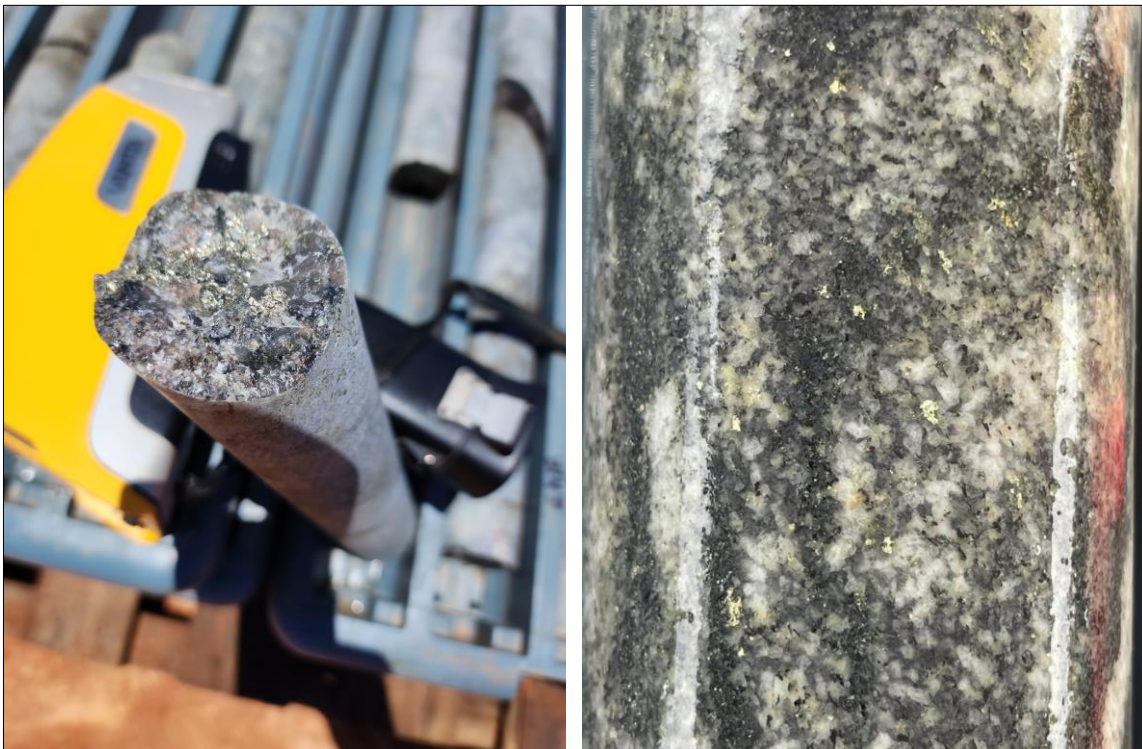
Figure 3: Visible disseminated sulphides within relatively fresh granite. Small golden blebs are chalcopyrite and silver-yellow sulphides are pyrite. These occur intermittently between 405 and 410m. Pyrite abundance is estimated to be about 3% and chalcopyrite about 0.5%.
