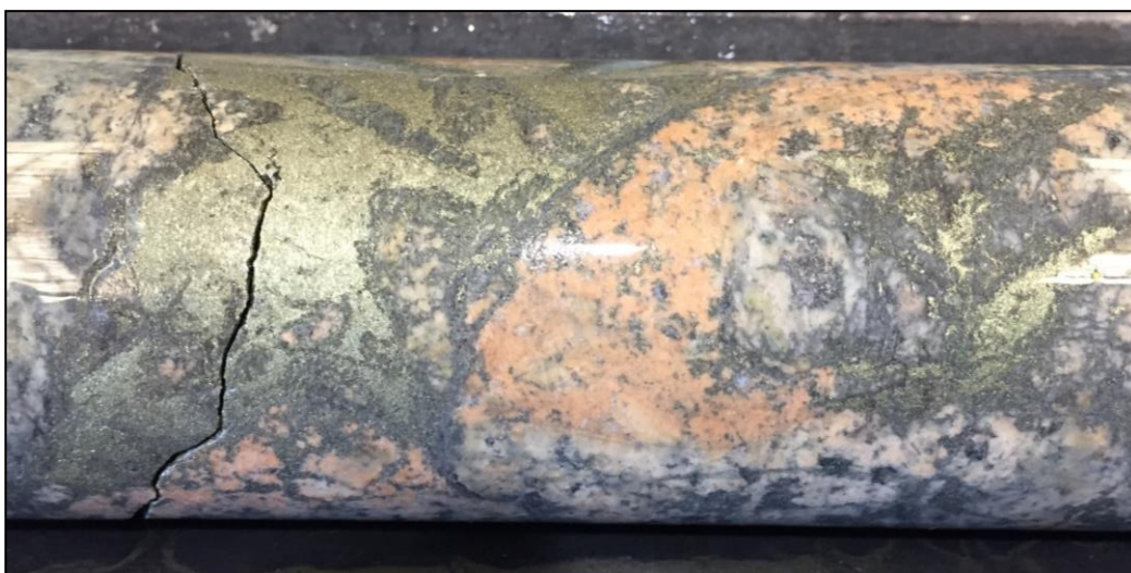
Figure 1. Breccia-hosted copper mineralisation west of the Corvette deposit, comprising 5.8 metres at 1.97% Cu & 179ppm Mo. This interval is one of the highest grade intersections ever drilled at the Myall Project (photograph from ~170 metres down hole in 23MYDD434, core diameter 45mm).
