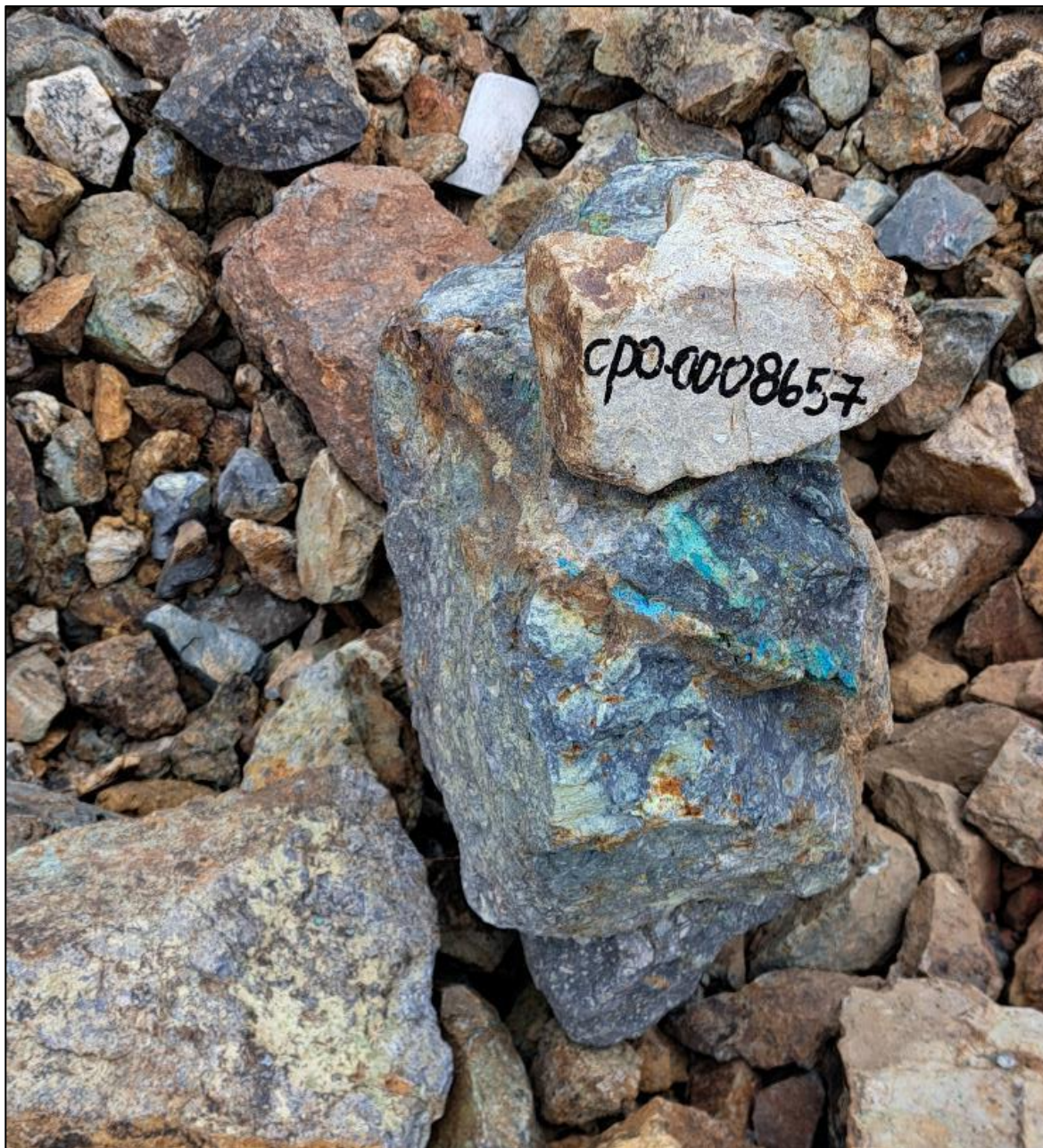
Figure 4: El Quillay North Stockpile sample CPO0008657 returned grades of 3.69% Cu.
