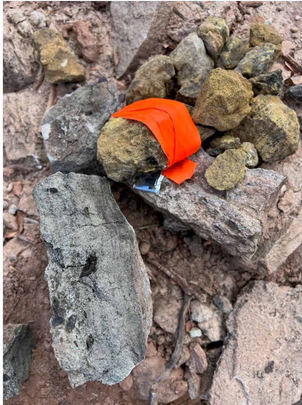
Picture 2: Carnotite (yellow) observed with possible uraninite or coffinite (black mineral) from the Stateline prospect. Location of this photo is Stateline with co-ordinate reading WGS84 UTM zone 12N 653129E 4214930N.
