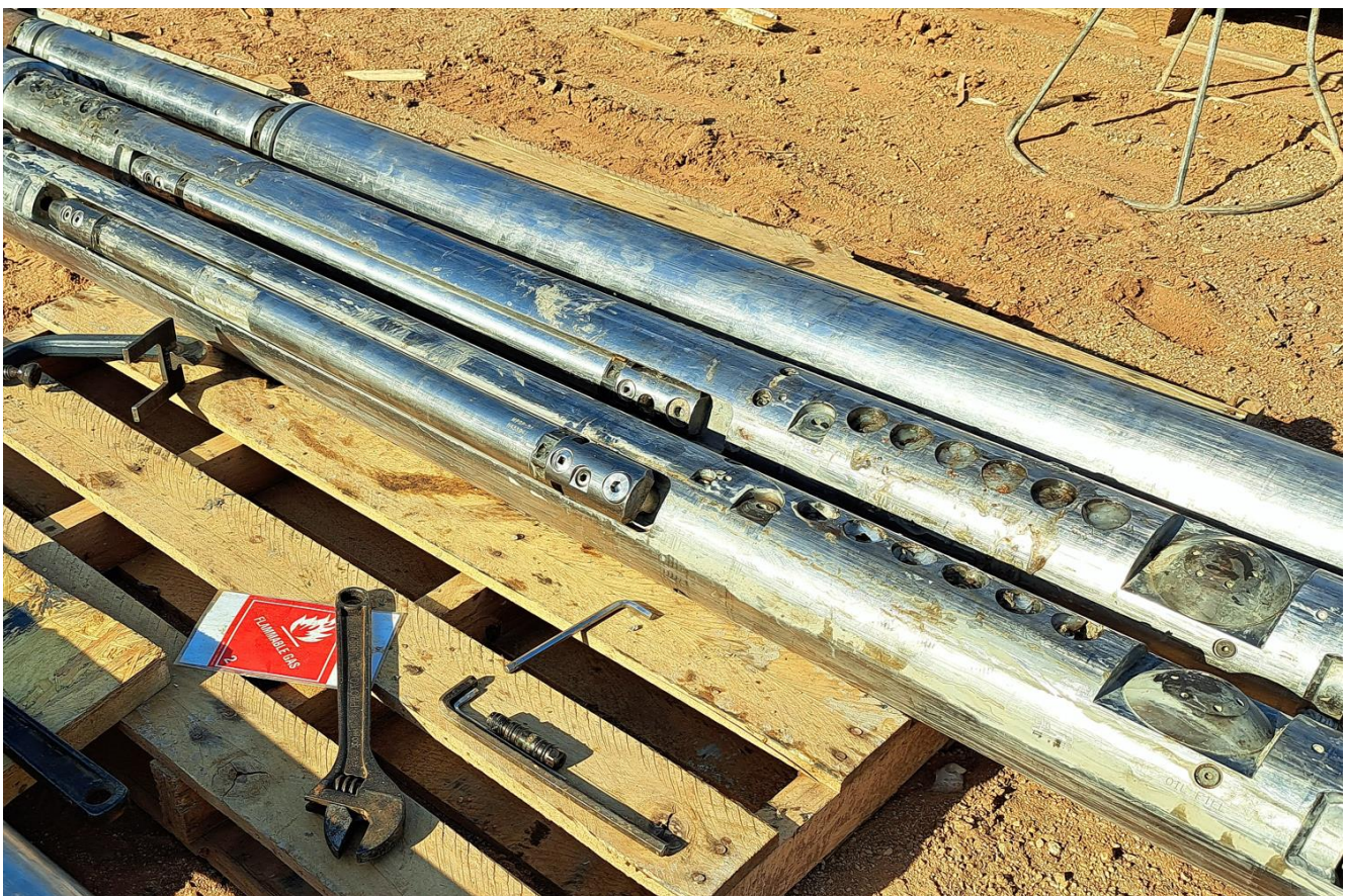
Figure 2 - Retrieval of pressurised sample chambers from the wireline formation testing tool at surface
