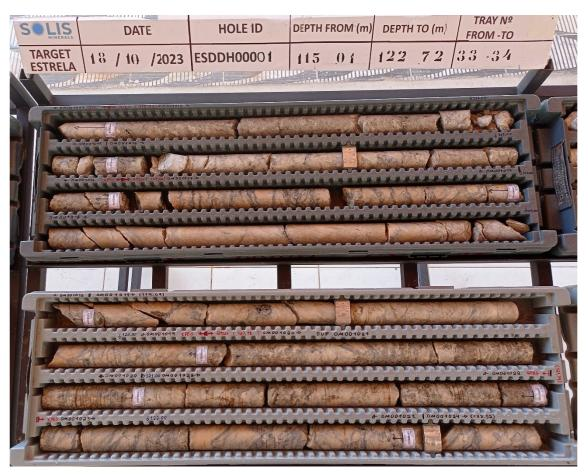
Figure 5: Pegmatite from Estrela drilling ESDDH00001 115.01m to 122.72m
