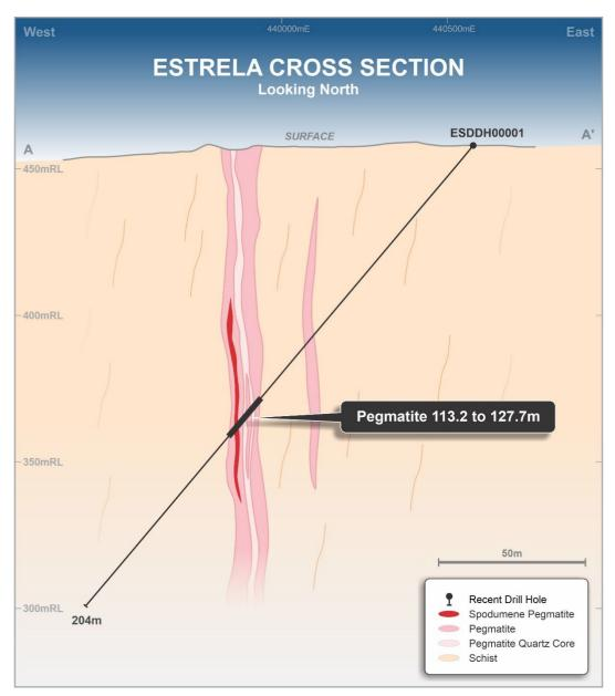
Figure 2; Estrela section showing ESDDH00001 and interpreted geology, 2 separate pegmatite bodies intersected.
