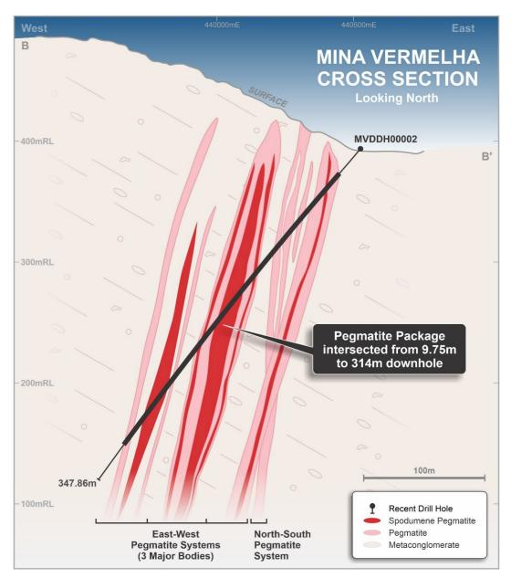
Figure 4; Mina Vermelha section showing MVDDH00002 and interpreted geology with multiple pegmatites intersected downhole, several pegmatites have been logged as containing visible Spodumene in trace quantities form 1-5%. Overall true width of mineralisation estimated at 48-75m
