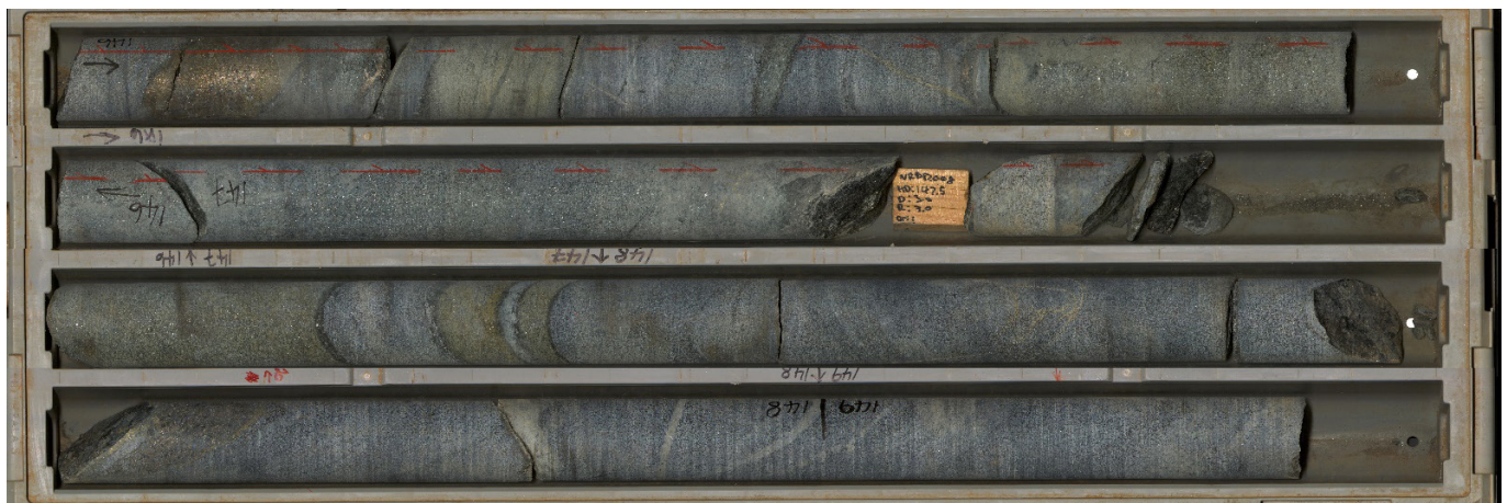
Figure 9 – Massive, semi-massive and disseminated sulphides hosted by mafic rocks intruded by minor felsic rocks contact with felsics and relevant excerpt from Table 1.
