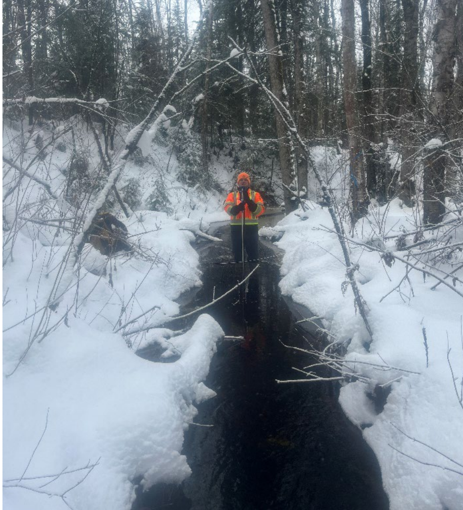
Figure 1 – Water flow measurements in local creeks, taken every season, to understand the water movement throughout the AOF.
