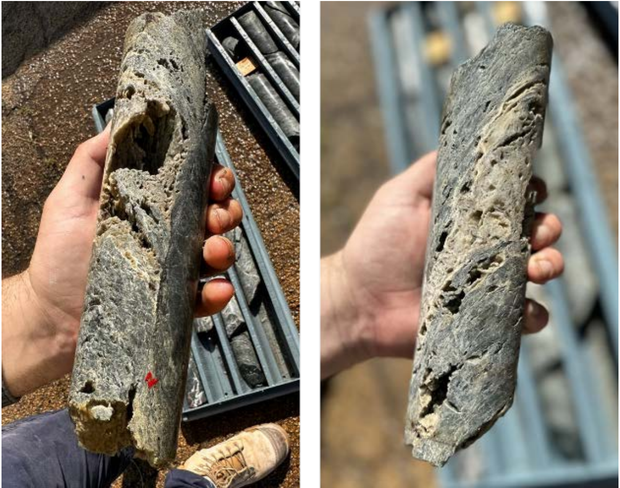
Figure 2: Drill core from 23LTRD001 showing cavities left after the dissolution of barite at 105.9m (left) and at 106.2m (right). A fracture parallel to the feeder fault zone can be seen in left photo.
