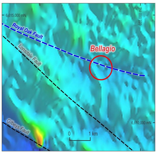
**Figure 5.** Bellagio Gold Prospect location located on the Royal Oak Fault, which can be traced on the Airborne Magnetic image (TMI) for over 20km within the Koonenberry Gold Project Area.
