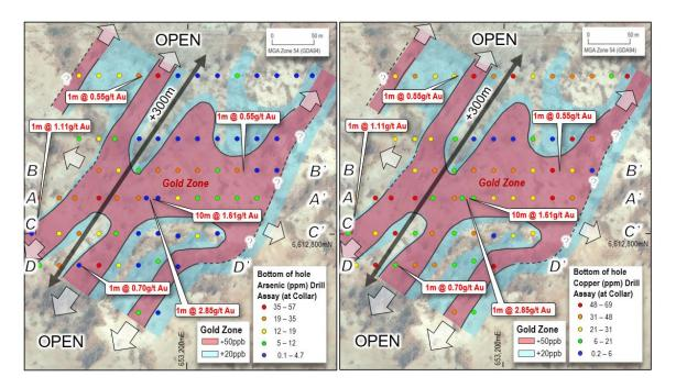
**Figure 4a.** Bellagio Gold Prospect showing bottom of hole Arsenic (ppm) with respect to plotted Gold Zones
