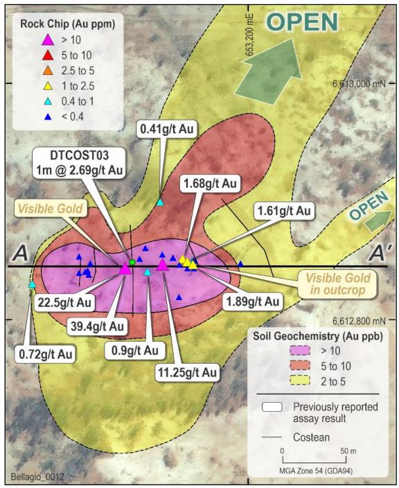
**Figure 3.** Bellagio Gold Prospect showing previously reported rock chip assays and gold in soil anomaly along with historical costeans over aerial photo.
