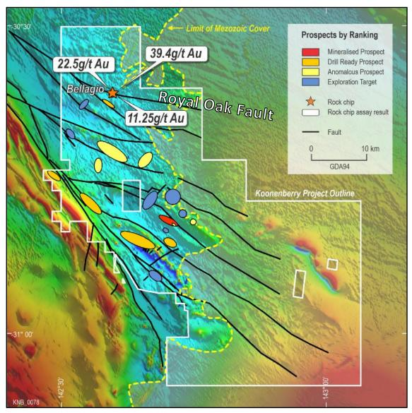
**Figure 6.** Koonenberry Gold Project with previously reported high grade rock chips at Bellagio, which is shown in relation to the 20km length strike of the controlling Royal Oak Fault.
