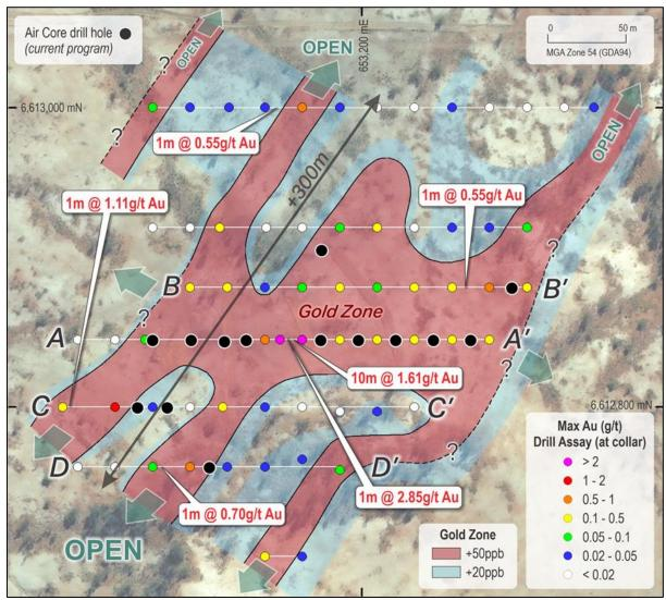
**Figure 2.** Plan view of the Bellagio Gold Prospect showing Phase 1 maximum down hole gold (g/t Au) at the drill collar. **Widespread gold mineralisation is observed over a 300m x 250m area and remains open both along strike to the NE-SW and laterally to the WNW-ESE.**
