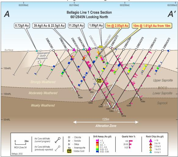
**Figure 1.** Cross section A-A' at Bellagio showing Phase 1 and Phase 2 drill hole traces with the latter targeting the gold zone below the Base Of Complete Oxidation (BOCO). Quartz veining associated with sericite-silica alteration has been intersected in the less weathered rocks across a 125m zone.
