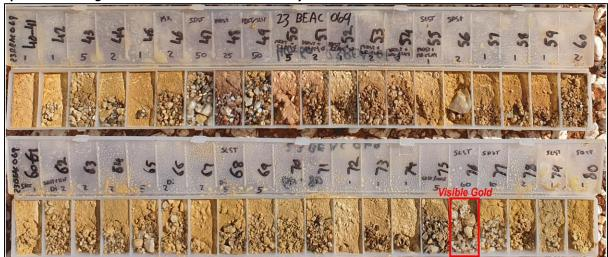
**Photo 1:** Chip trays from part of hole 23BEAC069, showing visible gold within a quartz vein (60% of the sample from 75-76m). Multiple flecks of visible gold were observed in the quartz chips and are of the order of 0.2mm in size each, possibly representing about 0.005% of the sample.
