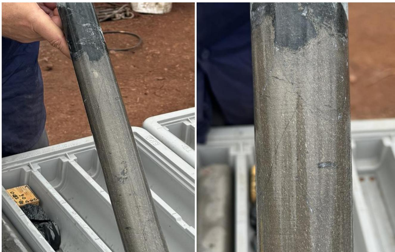
Figure 1: Massive sulphides within GYD040 at 279.85m
