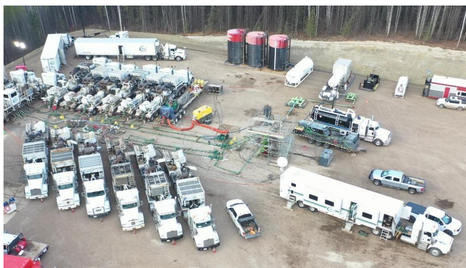
Figure 1: Frac spread on location at Gryphon Wapiti 16-02-65-08 well in North-Western Alberta, Canada.
