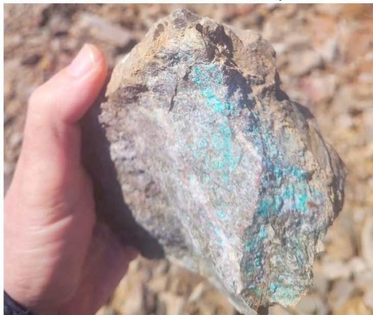
Figure 6: Ilo Este – porphyritic quartz microdiorite with potassic alteration and copper oxides in hand specimen from outcrop zone of high chargeability anomaly 4 . For location see Figure 7.
