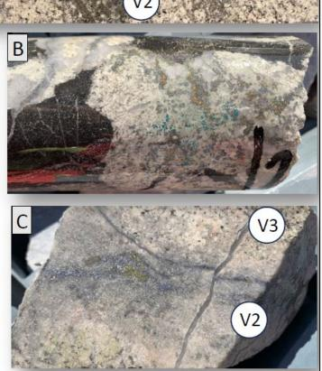
Figure 2: Core from CPW0002DD - V2 & V3 are two of three vein styles that appear to introduce the bulk of Cu & Mo (Wilson, 2023).
