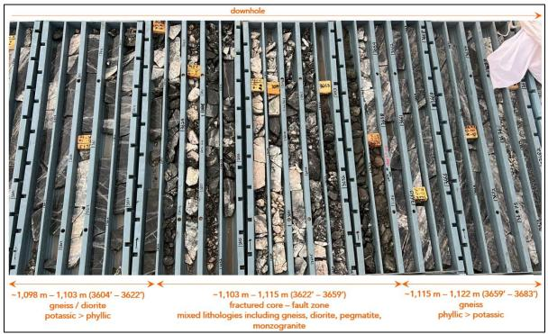
Figure 3: Cut core from CPW0002DD between 1,098 -1,120 metres depth showing the highly fractured zone which juxtaposes strong potassic alteration / Cu & Mo mineralisation (left) against pyrite-sericite-quartz dominated alteration (right)
