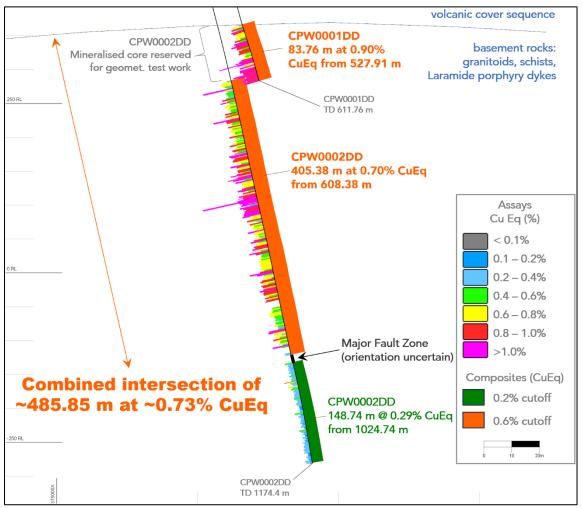
Figure 1: Cross section looking Northwest showing individual and composited assays at various cutoffs designed to represent the geological variability. Sampled overlap between the 0.6% CuEq cut-off intervals reported from CPW0001DD and CPW0002DD is 3.29 metres. The two holes are approximately 14.65 metres apart at the TD of CPW0001DD (V/H = 1/4).
